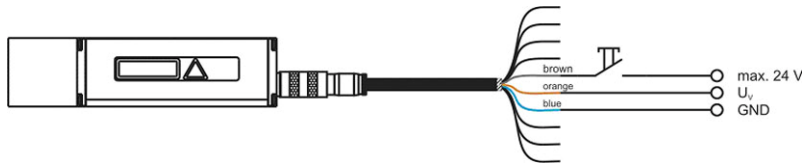
Figure 22: Wiring diagram of trigger input
