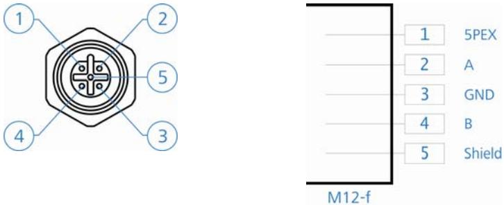
Figure 7 Profibus-OUT connection diagram
