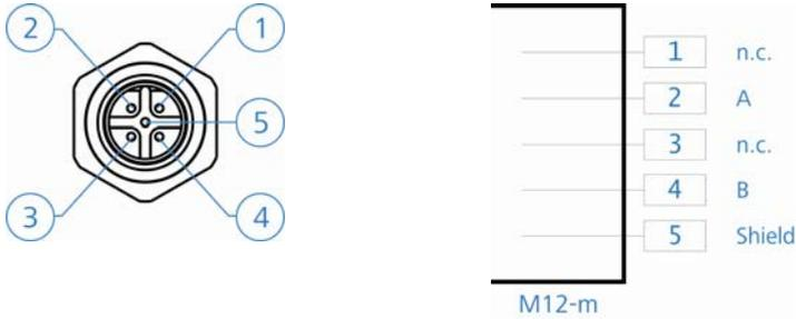
Figure 6 Profibus-IN connection diagram
