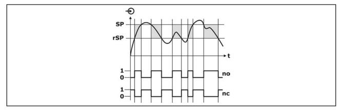
The window function realizes a signal range – acceptance region –, where the switch output is set to a definitive switch state.
