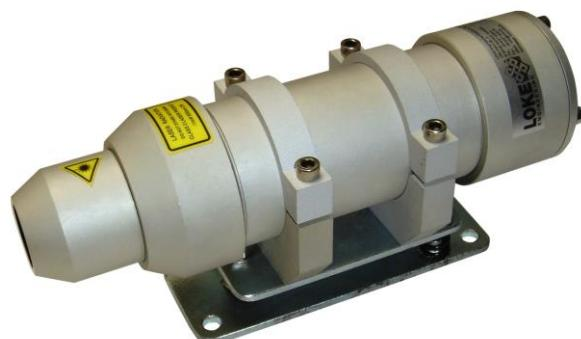
The laser distance meter LMC-J-0060 is robustly engineered especially for industrial applications. It works on reflector at distances up to 500 m. Up to 100 m (depending on target reflectivity) no special reflector is needed. Measuring values are provided continuously via the integrated interface RS232 / RS422 / 485 and analogue output 4... 20 mA.
