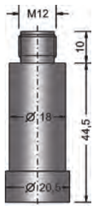
connection housing electronics output type A / E - 2-wire, signal 4...20mA
