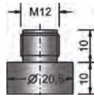
connection housing electronics output type B / C - Pt100, 4-wire
