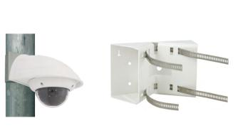
Installation of the Vandalism Kit (Accessory) Screw in the reinforced dome and set the four spacers onto the mounting ring of the camera. Place the stainless steel outer shell onto the camera
