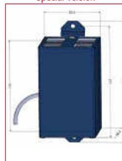
Wiring cable and screw mounting vertical
