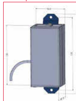
Wiring cable and screw mounting vertical
